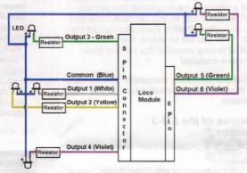
WARNING: Using LED's without resistors can damage the LED's! Use 1k Ohm 1/4W for 15mA or 750 Ohm 1/2W for 20mA. WARNING: If you use the wrong resistor, it is possible to generate enough heat to ignite flammable material, and possibly cause a fire.
